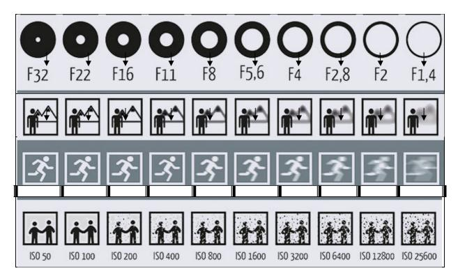
The diagram shows the relationship of: aperture, shutter and ISO. In the blank spaces, give the corresponding shutter speed settings from these: 1/2; 1/125; 1/30; 1/250; 1/1000; 1/15; 1/4; 1/500; 1/8; and 1/60. **[10]**
