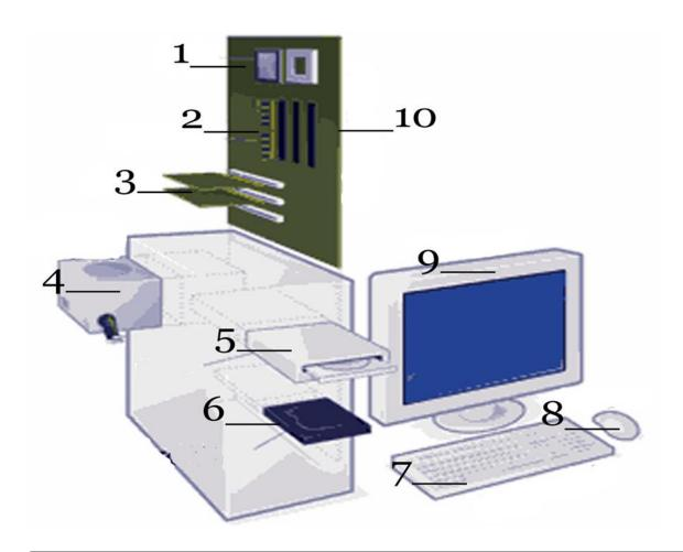
Keyboard, Power Supply, CPU (Microprocessor), Motherboard, Monitor, Expansion cards, Secondary storage (Hard disk), Primary storage (RAM), Mouse, Optical disk drive
